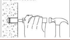
Using the tool, set the anchor by driving the lead sleeve over the cone using several sharp hammer blows. Be sure the anchor is at the required embedment depth so that anchor threads do not protrude above the surface of the base material. Positions the fixture, insert screw or bolt and tighten.
